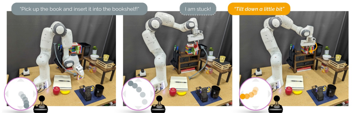
Figure 2: A user interacts with our system. [Left] The user utters “pick up the book and insert it into the bookshelf,” inducing a low-dimensional controller (depicted with the joystick and shaded inputs). [Middle] This control space is state and language-conditioned: pressing down brings the end-effector close to the book, while holding up/left after grasping the book moves the end-effector towards the shelf. However, this static controller is not enough; the user gets stuck! [Right] Our approach allows users to provide real-time corrections (“tilt down a little bit”) refining the control space so the user can complete the task.
