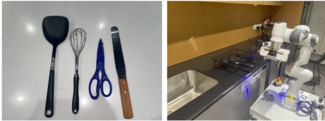
Fig. 5: (Left) Utensils used for the experiment: spatula, egg whisk, scissors and knife. (Right) The experiment environment that emulates a kitchen.
