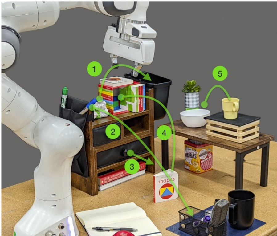
Figure 5: Setup of our tabletop manipulation environment with sketches of our high-level tasks (further details in §5).
