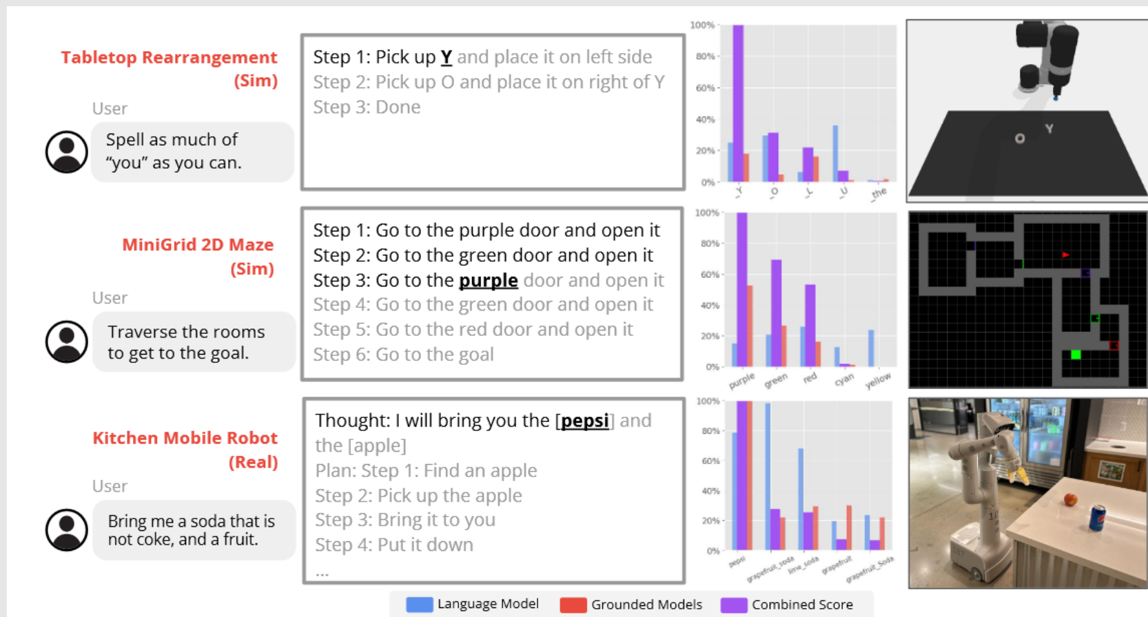
Figure 3: Example rollouts and likelihood of representative tokens under Grounded Decoding objective in three distinct domains: simulated tabletop rearrangement ( top ), Minigrad 2D Maze ( middle ), and real-world kitchen mobile manipulation ( bottom ). Each domain uses different prompts, grounded models, and low-level primitives. The GD formulation is shared across the domains, decoding a pre-trained language model with respect to domain-specific grounded models to decompose a open-ended instruction into actionable steps.
